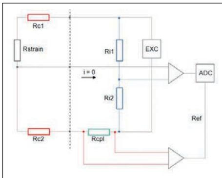
**Fig. 3: Gantner Instrument's three-wire circuitry with compensation of cable influences**
