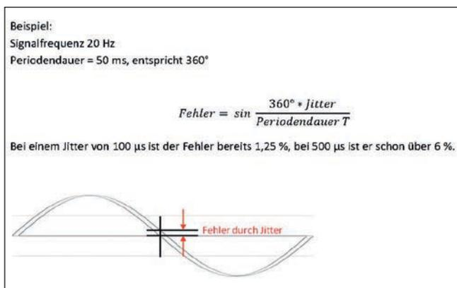
**Fig. 4: Influence of non-exact synchronized measurement data: Jitter of only 1 microsecond in the Q.bloxx A116 strain-gauge module causes negligible influence of 0.0125%.**
