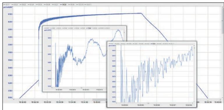
Fig. 1: Increase in load up to destruction of the blade
