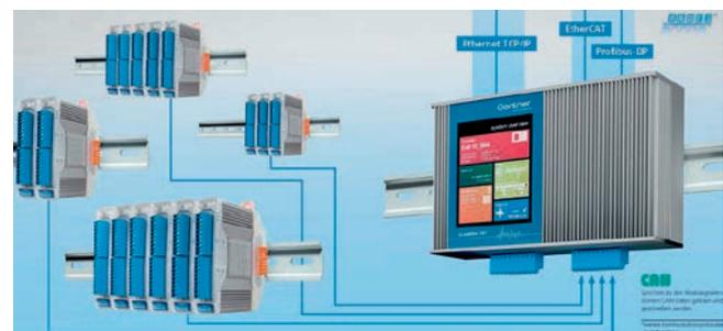
**Fig. 5: Configuration of a measurement system with up to 500 channels based on Q.series instrumentation**
